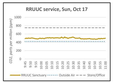
Carbon dioxide monitor readings (above) taken in the Sanctuary during a recent Sunday service show concentrations (500 ppm) close to that of outdoor air (420 ppm). For comparison, indoor CO2 levels are typically 700 to 800 ppm in commercial buildings. Ongoing CO2 monitoring at RRUUC helps us verify that our building is well-ventilated—a critical component of infection control.
